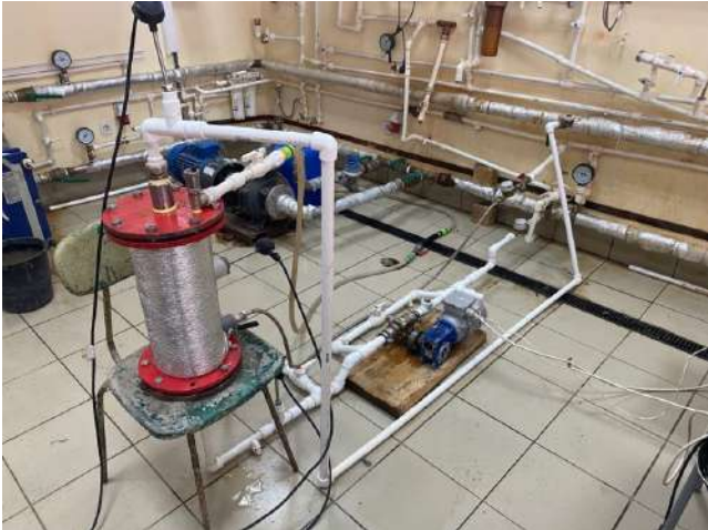
Figure 7: Experimental Setup for Testing a Capacitive Heat Exchanger with an Oscillating Coil.
